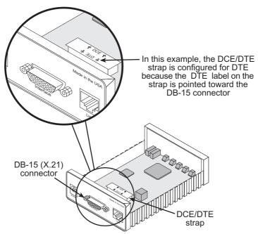
Figure 10. Setting the DCE/DTE strap
